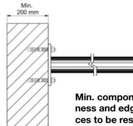
Min. component thickness and edge distances to be respected
